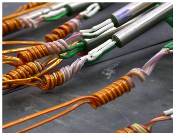
5. Thermocouples 'interruption' with Kapton connection
