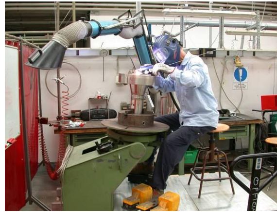
2. Safety chamber GTAW qualified welding
