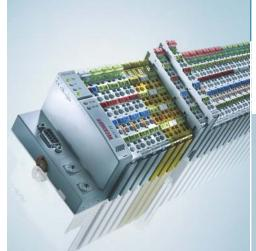
TwinSAFE: safety technology directly in the I/O system
